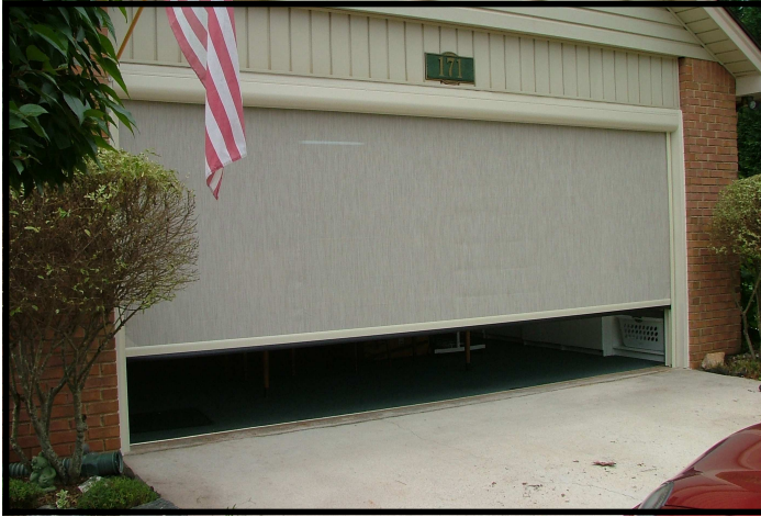
(pictured above) INSIDE UNDER HEADER (IUH): Hood mounts inside the opening, under the header. Tracks mount inside the opening, between the jams.
