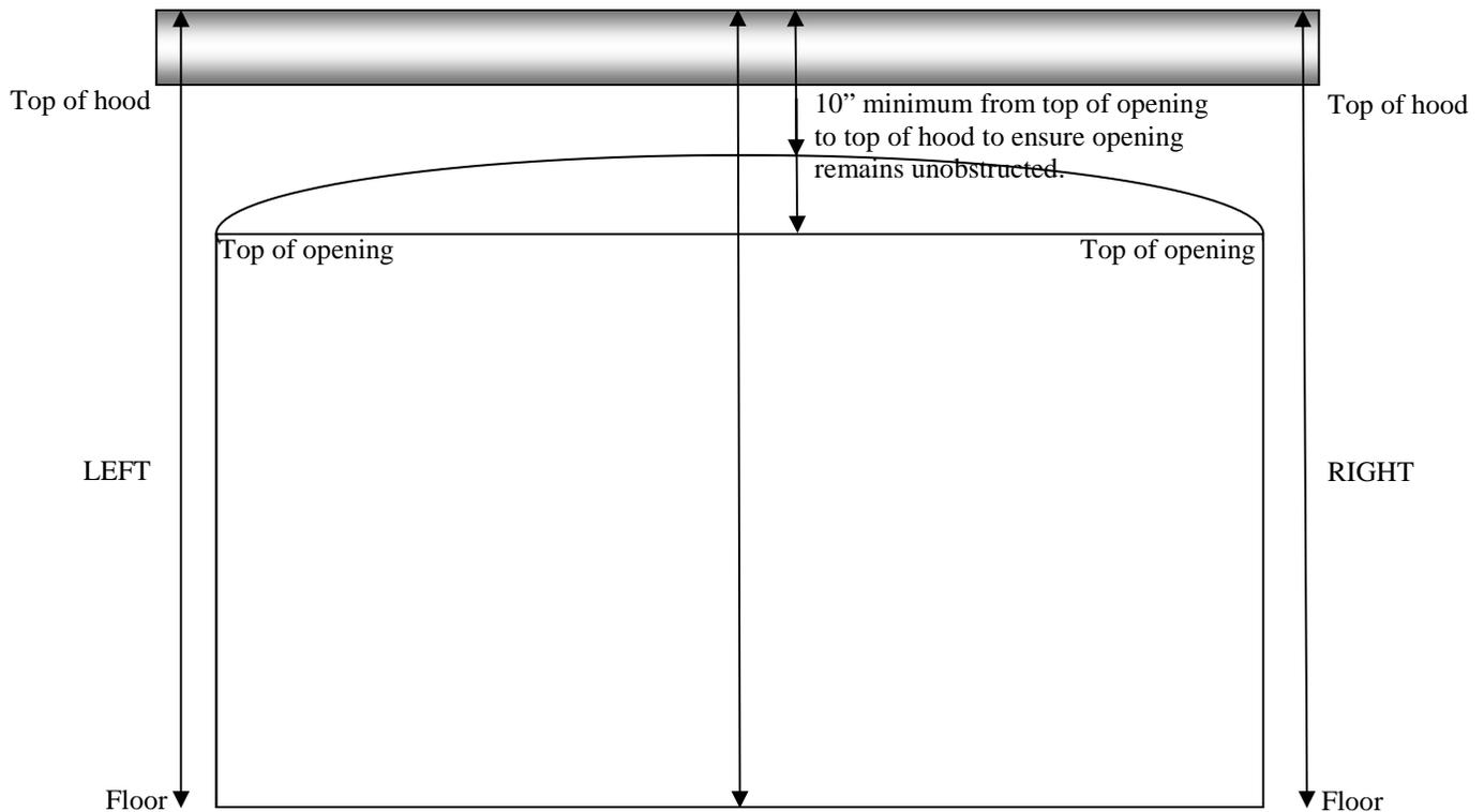
ABOVE: For **OAH** install (outside above header), take a 3 point measure on the extreme left, center, and extreme right. Measure from floor to top of hood. Note any differences in height. Add at least 10" if you want to ensure the opening remains unobstructed. Use this type of installation for arched openings.
