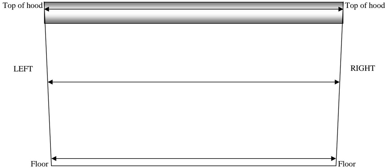
ABOVE: For IUH install, top is wider than bottom. Take a standard 3 point measure at the top, middle, and bottom of the opening. If variance is less than 1", note on order sheet. Use the angle for the adjustments on the tracks during installation. If over 1" variance, call for instruction.
