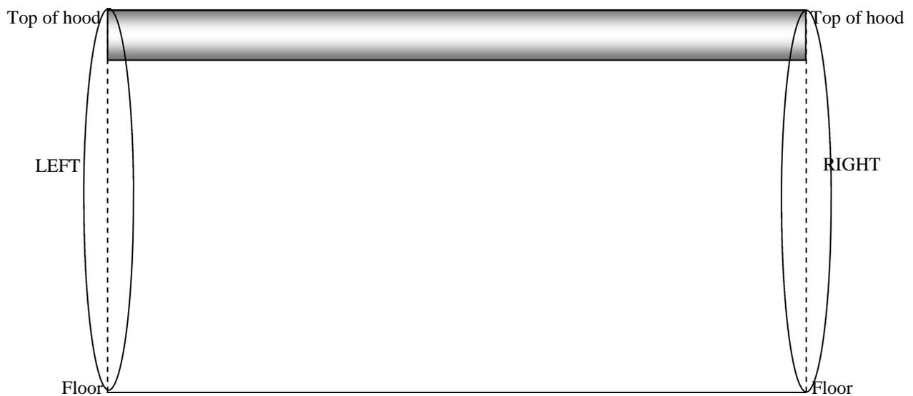
ABOVE: For IUH install, the jams bow out or in on the sides. Take a standard 3 point measure at the top, middle, and bottom of the opening. If variance is less than 1", note on order sheet. Use the angle for the adjustments on the tracks during installation. If over 1" variance, call for instruction. You will most likely have to either shim out the jams, or use caulk to seal the open spaces once install is complete. Header must be level!
