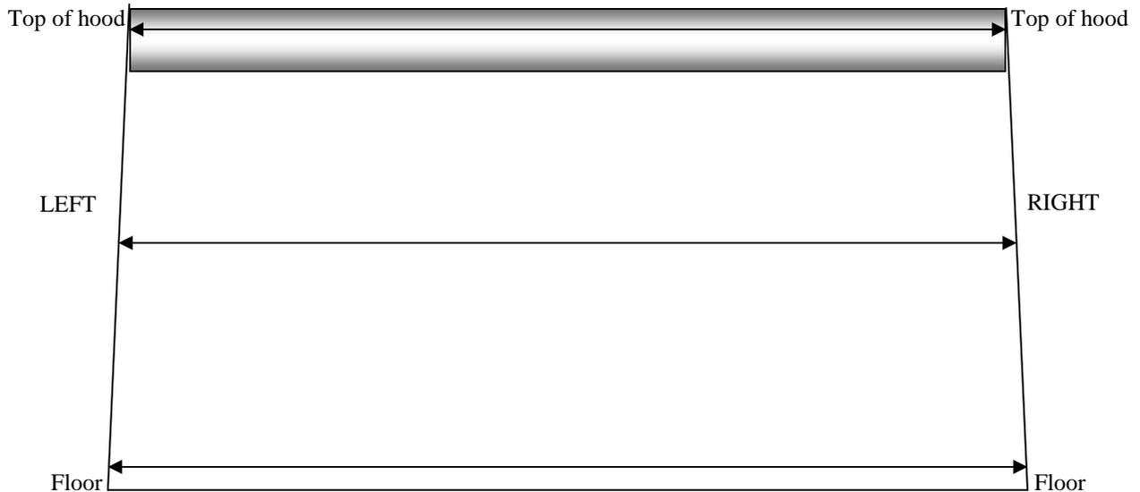
ABOVE: For IUH install, bottom is wider than top. Take a standard 3 point measure at the top, middle, and bottom of the opening. If variance is less than 1", note on order sheet. Use the angle for the adjustments on the tracks during installation. If over 1" variance, call for instruction.
