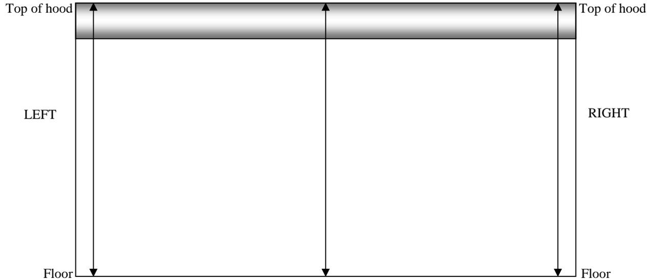
ABOVE: For **IUH** install (inside under header), take a 3 point measure on the extreme left, center, and extreme right from floor to top of hood. Measure while facing **ROUND** part of the hood.. Note any differences in height. Header must be level! For recessed install, measure from floor to top of bracket on left and right sides.
