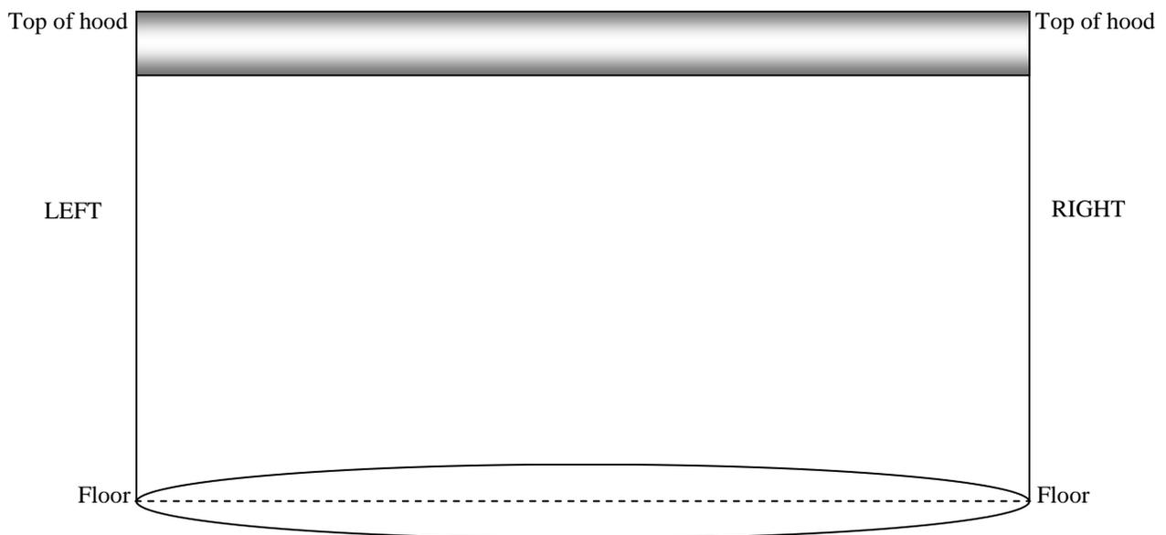
ABOVE: For any install, the floor dips in center or has a bump in the center. Bug rubber and felt can only accommodate about a 1/2" variance. You will have to either level out the ground, or let your customer know that there will not be a tight seal at the bottom due to uneven surface. Header must be level!
