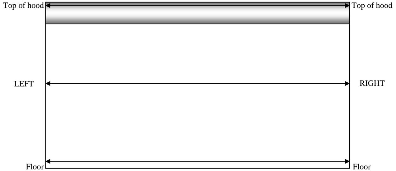
ABOVE: For **IUH** install (inside under header) and recessed applications, take a 3 point measure at the top, center, and bottom of the opening while facing the **ROUND** part of the hood (front of unit). Note any differences in width. Tolerance up to 1" variance. For recessed installation, measure from where the back of the bracket will be to the back of the other bracket, and deduct 1/4" for play.
