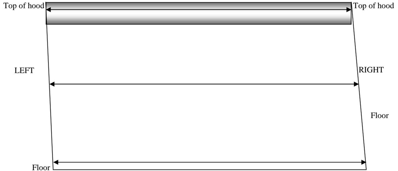
ABOVE: For IUH install, opening is a parallelogram. Take a standard 3 point measure at the top, middle, and bottom of the opening. Use a level on the sides and you will need to frame out the sides to make the jams square. Header must be level!
